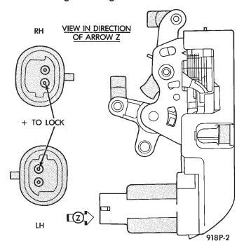
Fig. 3 Front Door Lock Motor
