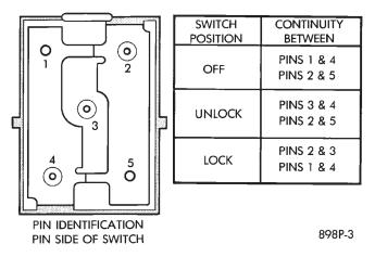
Fig. 1 Door Lock Switch Continuity
