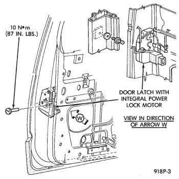
Fig. 5 Front Door Assembly
