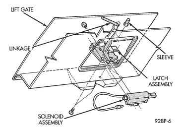
Fig. 4 Lift Gate Release Assembly
