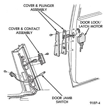
Fig. 6 Sliding Side Door Wiring and Component Identification
